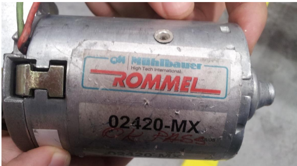
Fig.4.22 Motor DC 24V, 140 rot/min
