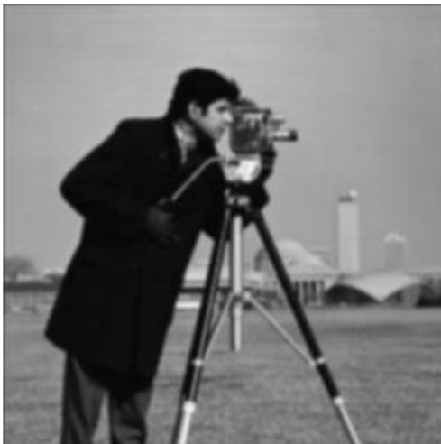
Filtru Gaussian 11x11 sigma 1
